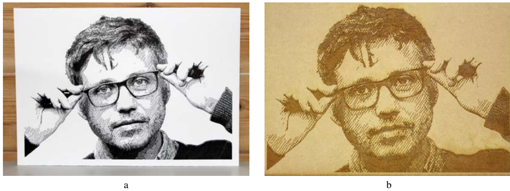
Figure D.17: Crosshatching drawing made with the LinesLab system. (a) The illustration is drawn on paper (b) The same illustration etched on MDF with a laser cutter
