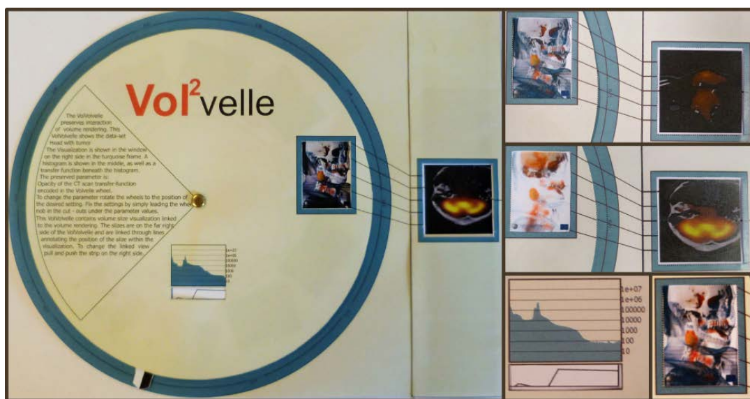
Figure B.18: Finished Vol 2 velle with linked views. The slice position is indicated through lines. Rotation of the wheel changes the opacity and updates the linked transfer function as shown on the lower right.
