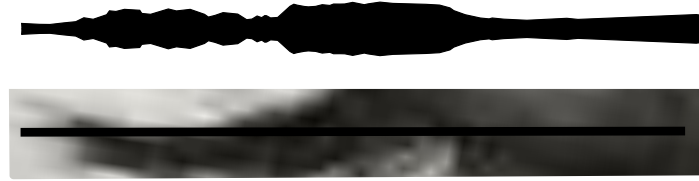
Figure D.12: The shape of the polygon encodes the darkness values along its centerline as thickness.
