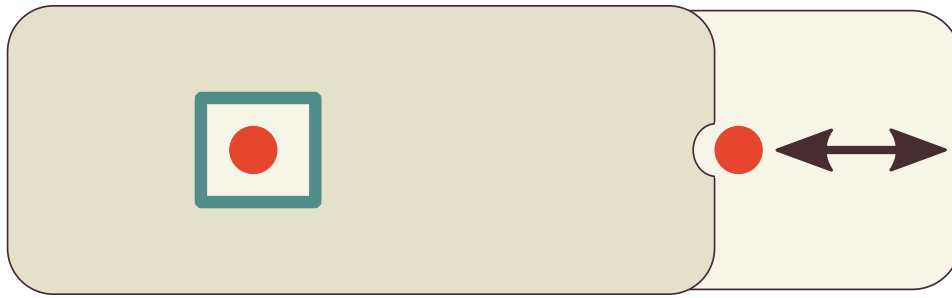
Figure 3.11: Interactive charts do not require circular layouts. A slide chart is able to encode one-dimensional interaction with an envelope-like cover and an information chart that can be pushed through.
