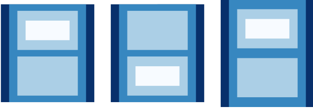
(a) One-dimensional treemap over time. The white rectangle changes its parent element from step 1 to step 2. Between step 2 and step 3, the white node is deleted and a new white node is created. These hierarchical changes are not visually distinguishable.
