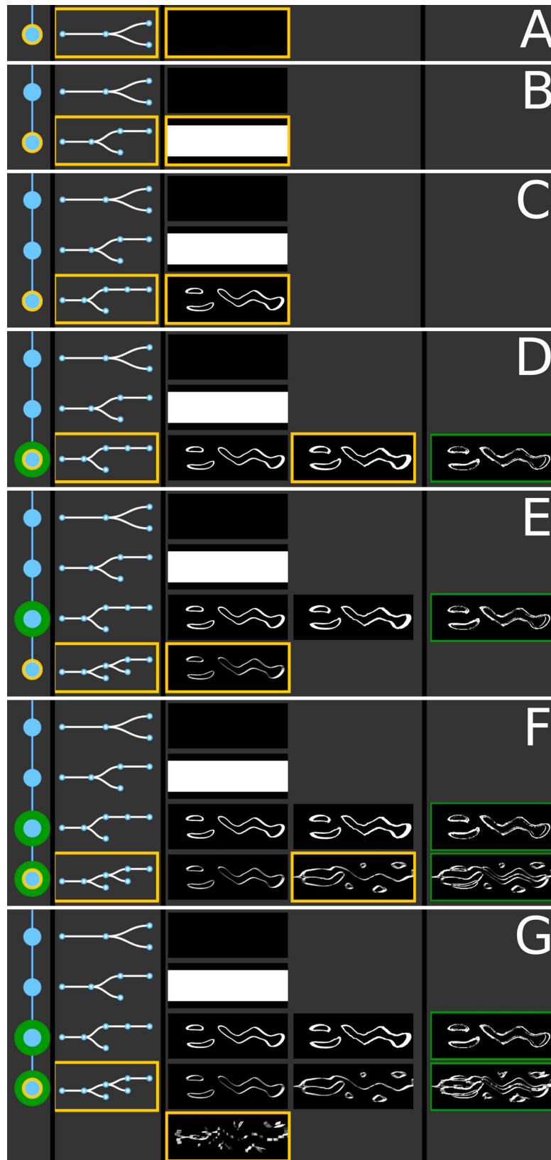
Figure B.7: Visualization of a visualization source code evolution. (A) Initial state. (B) Implement ray tracing and find volume. (C) Implement flow visualization based on flow magnitude. (D) Test trilinear interpolation instead of B-spline interpolation. The comparison image highlights minor differences. (E) Implement shading. (F) Change the flow feature from flow magnitude to extremum lines. (G) Test trilinear interpolation instead of B-spline interpolation.
