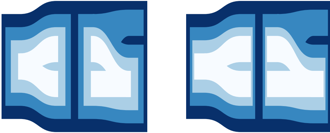
Figure C.3: Left: Hierarchical Margin. Streams receive a higher margin, the deeper their hierarchy level is. Right: Reversed Hierarchical Margin. Streams closer to the root receive larger margins. Although both cases feature the same margin on the root node, the latter case provides a clearer representation of changes over time, because leaf nodes are not pushed so far away from each other.
